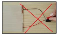
Don't pull the busbar wire, the busbar is easy to pull separate with the film or glass! Import! If there have some water or alcohol on the busbar and film edge position, don't connect power, let the film dry totally, then connect the power!
